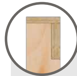
Notched stud with continuous lintel
